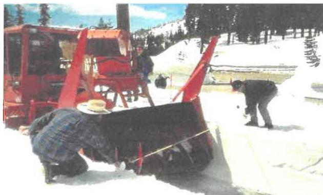
**FIGURE AI** - Measuring the Rotary Plow's Width and Depth Pass When Employing the Field Testing Method
