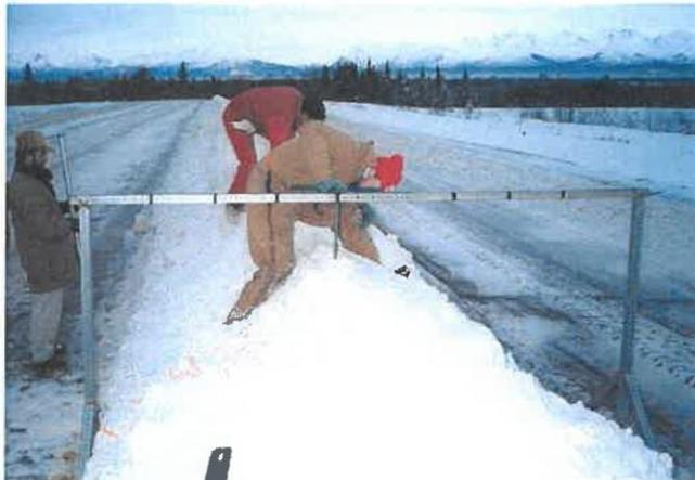
**FIGURE A4** - Measuring the Windrow Using a Gantry When Employing the Constructed Windrow
