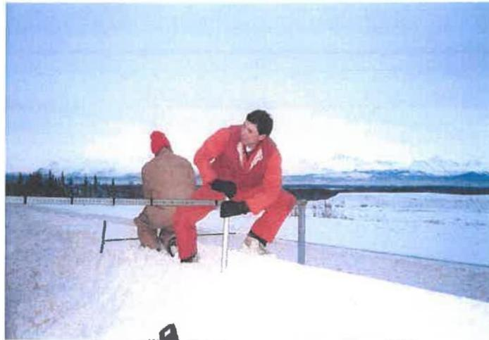
**FIGURE A5** - Using the Coring Tool on Constructed Windrow
